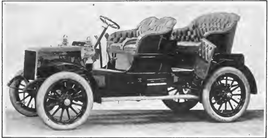
NEW WINTON CAR WITH FOUR-CYLINDER TRANSVERSE MOTOR IN FRONT.
